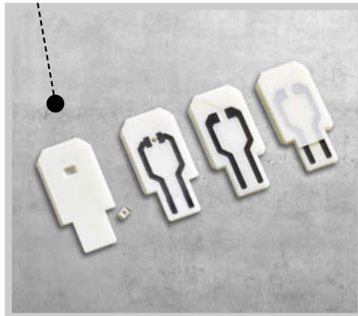
Conductive material compound (ABS with carbon nano tubes): direct contacting of a manually inserted LED.
