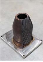
Combustion Chamber SS316L – Aerospace
