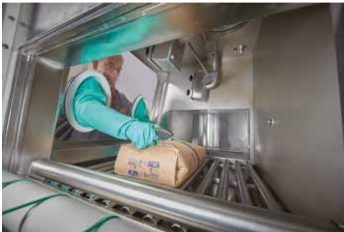
Glovebox with two-hand safety control unit and integrated blade for opening the bags
