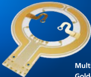
Bondable \text{Al}_2\text{O}_3 -Substrate with 100 nm Flash-gold
